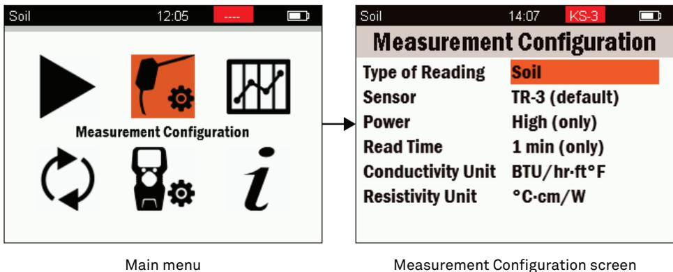
Figure 5 Navigate to the Measurement Configuration screen
